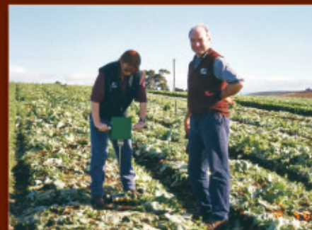
Measuring soil compaction with a penetrometer
